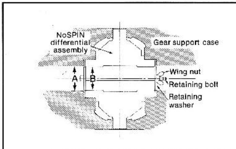
The bolt washers and wing nut used to retain the NoSPIN differential assembly when it was shipped from the factory as illustrated on page 13, are best for this purpose. You will note that the retaining washers must be small enough to pass through the case ends (dimension "A"), yet large enough to restrain the two side gears (dimension "B") and the balance of the NoSPIN differential assembly when all parts are assembled and the springs are compressed.
