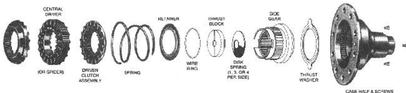
Note the additional parts compared to NoSPIN/Detroit locker differentials, page 5. New IMPROVED Detroit Locker models are supplied with either a spider or central driver and a support case.
