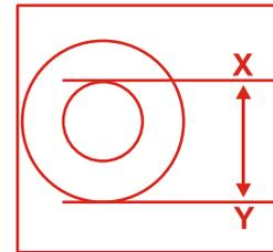
The diameter of the tires can be adjusted by varying the air pressure of the tires.
